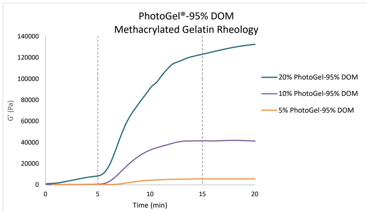
Figure 1. A compilation of the viscoelasticity graphs of PhotoGel at concentrations of 5%, 10%, and 20%. Dashed lines are used to mark the beginning of the 405 nm light exposure at 5 min and the end of that exposure at 15 min.
