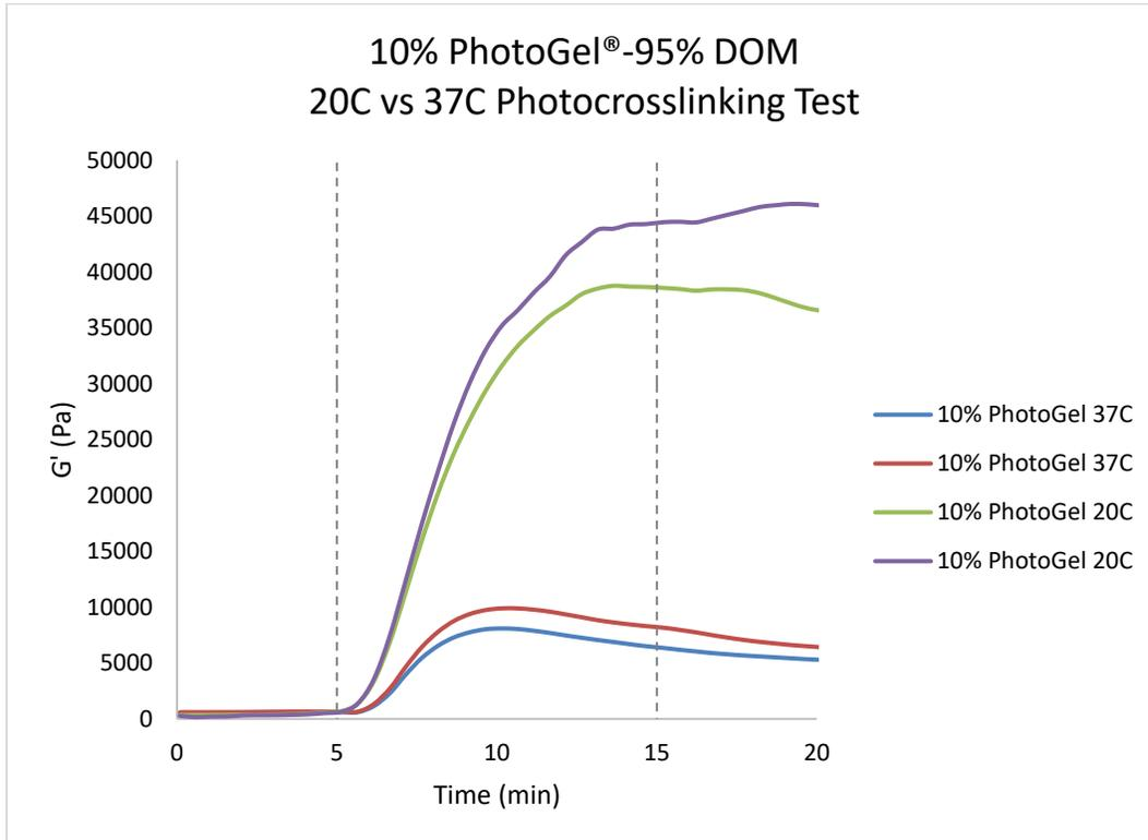
Figure 2. A compilation of the viscoelasticity graphs of 10% PhotoGel at temperatures 37C and 20C. Dashed lines are used to mark the beginning of the 405 nm light exposure at 5 min and the end of that exposure at 15 min.
