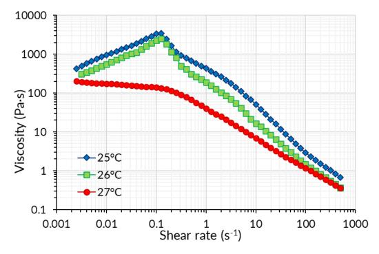
**Figure 1.** Viscosity change of GelMA Bioink upon applied shear forces at various temperatures over a shear rate range of 0.01 to  $500 \, \text{s}^{-1}$ .
